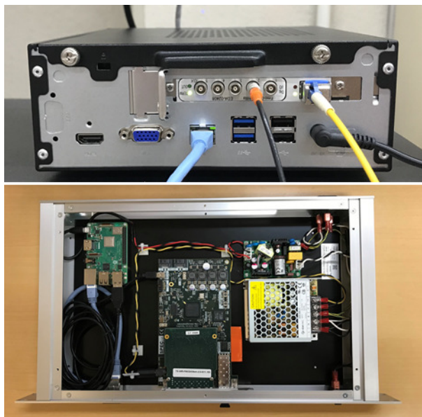
Figure 1: Pictures of the slave node: the upper picture is SPEC on the homebuilt computer. In the lower picture, SPEC is housed in the 19-inch box with 1U height. It can be operated from RaspberryPi.
