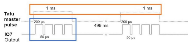
Figure 3: The port IO7 producing output pulses at the master pulse pace.
