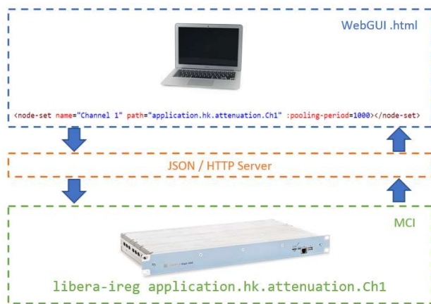
Figure 4: HTTP REST API application architecture node detail.
