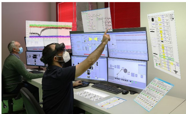
Figure 2: Panels in AR added as additional virtual desktop in the main control room.
