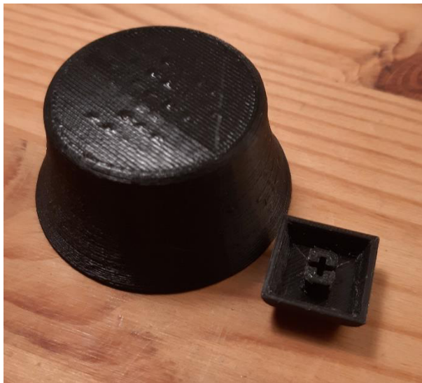
Figure 2: Mechanical parts realized with FDM technology.
