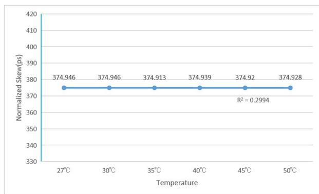
Figure 12: Result of the temperature drift test.
