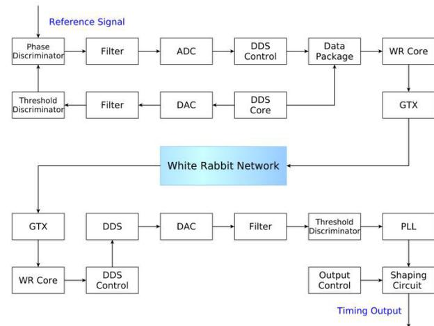
Figure 6: Prototype II system architecture.
