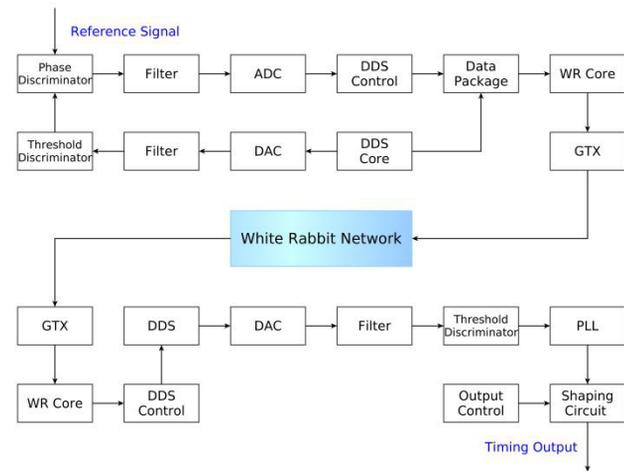
Figure 6: Prototype II system architecture.
