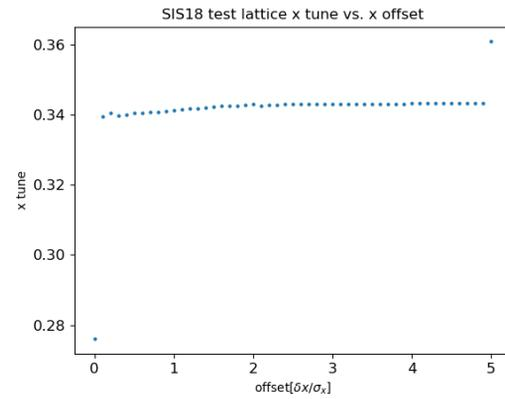
Figure 7: Tune depression ( $x$ ) vs original  $x$  offset for a varying number of physical and macroparticles. In Fig. 6,  $N_{physical} = 6.4 \cdot 10^6$ ,  $N_{macro} = 6.4 \cdot 10^6$ , whereas here  $N_{physical} = N_{macro} = 6.4 \cdot 10^4$ . Note how using too few physical particles (or inappropriate macroparticles) fails to capture the appropriate behavior.
