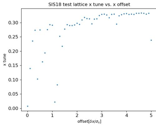
Figure 6: Tune depression ( $x$ ) vs original  $x$  offset for modified interaction kernel ( $1/(r + \delta)$ ) using simulations with  $6.4 \cdot 10^6$  physical particles and  $6.4 \cdot 10^4$  macroparticles. In Fig. 5,  $\delta = 10^{-2}$  was set while here, we set  $\delta = 10^{-5}$ . Note how less regularization leads to a much noisier outcome.
