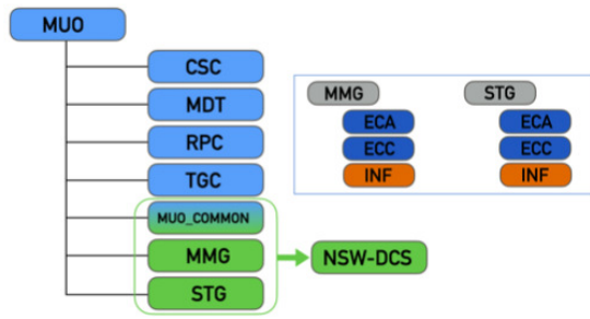
Figure 1: The overview of the ATLAS MUO DCS FSM structure with NSW DCS integration and brief structure of the sub-detector node structure.
