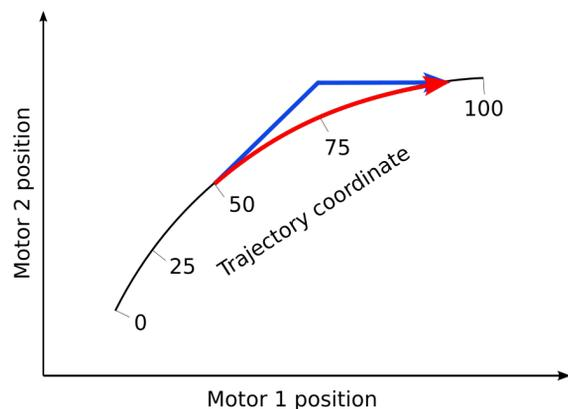
Figure 1: The difference between typical pseudomotions and parametric trajectories for a move along the parameter axis. The pseudomotor starts moving both motors at their nominal velocity. Once the first motor has reached its position, the second continues moving towards the target. The parametric trajectory on the other hand follows the trajectory the whole way by continuously adjusting the motor velocities.
