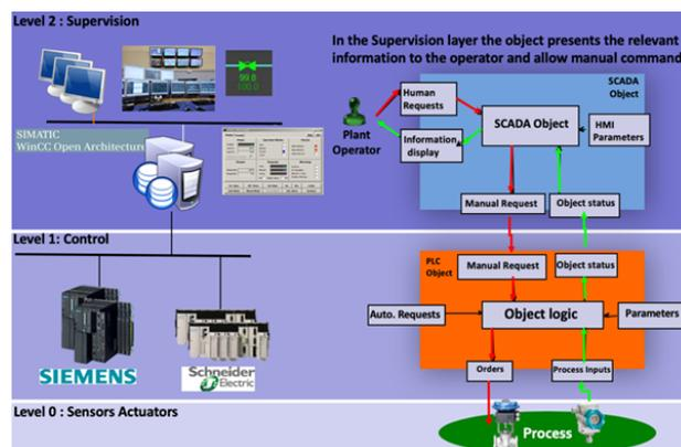
Figure 3: UCPC Control & supervision layer integration.
