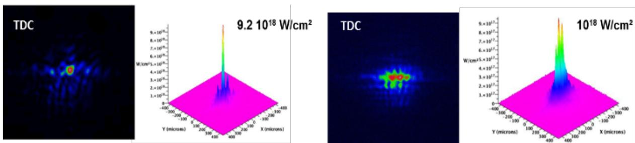
Figure 3: Focal spot (left) for the 358 J @ 690 fs shot giving  $9.2 \times 10^{18}$  W/cm<sup>2</sup>, focal spot (right) optimized for the shot on the 25 μm wire with 396 J @ 3 ps and  $10^{18}$  W/cm<sup>2</sup>. They are measured on the compression diagnostic table TDC during shot.
