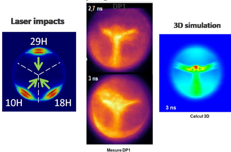
Figure 5: Hydrodynamics measurement of the cavity walls.
