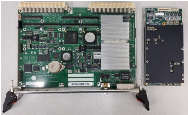
Figure 5: MVME3100 and PENTEK7142 for Linac BPM.
