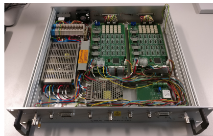
Figure 4: Custom pre-amplifier box developed at LNL.
