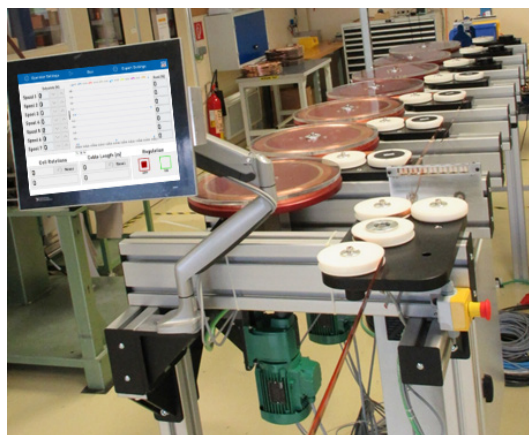
Figure 4: Winding machine with touch-panel user HMI.
