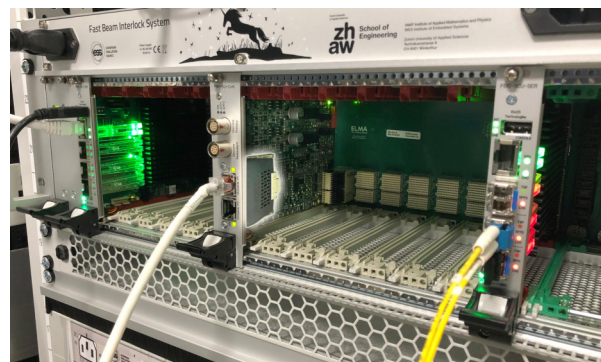
Figure 4: Highlighted the Anybus mounted on the MC. On the left and right of the crate the two cards where the Zynq® UltraScale+™ MPSoC XCZU7EG-FFVF1517 are mounted.
