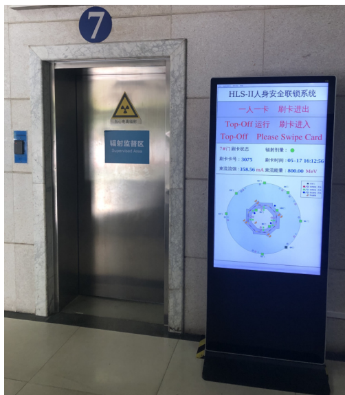
Figure 5: Photo of the novel HLS-II PSS Door Display OPI.
