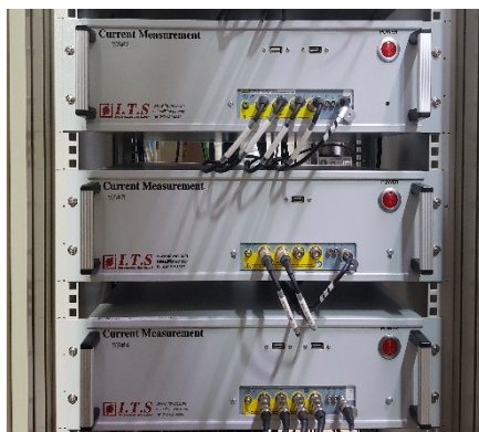
Figure 5: The wire scanner control units installed at KOMAC linac.
