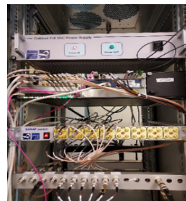
Figure 2: RF cabinet with MTCA LLRF crate.
