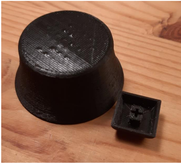
Figure 2: Mechanical parts realized with FDM technology.
