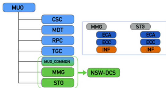
Figure 1: The overview of the ATLAS MUO DCS FSM structure with NSW DCS integration and brief structure of the sub-detector node structure.
