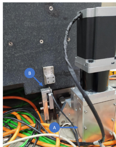
Figure 2: Leveller actuator (A) and feedback encoder (B).
