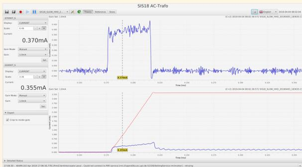
Fig. 4: Transmission monitoring of UNILAC beam, here 40µs macro-pulses (top) to SIS18 synchrotron. Red curve shows the ideal efficiency, blue bottom graph shows the measured increase of intensity in the ring.
