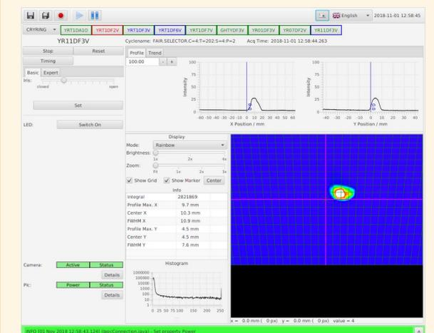
Fig. 9: Video imaging with CUPID for beam profile measurement on scintillating screens
