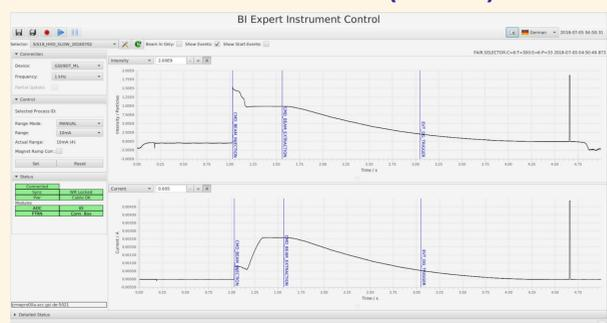
Fig. 5: Intensity plot in number of particles (top) and beam current (bottom) in SIS18 using a DCCT.
