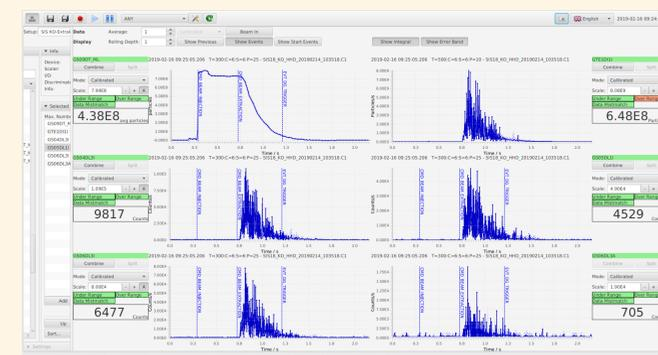
Fig. 8: Synchronous visualization of different acquisition types (ADC, scaler) in LASSIE of a complete SIS18 cycle. Upper left: Intensity in SIS18 (ADC). Upper right: slowly extracted beam in HEBT on plastic scintillator. All others graphs are in-ring beam boss monitors.
