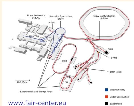
Fig. 2: Scheme of existing GSI (blue) and the new FAIR accelerators (red) plus attached experiments (black)
