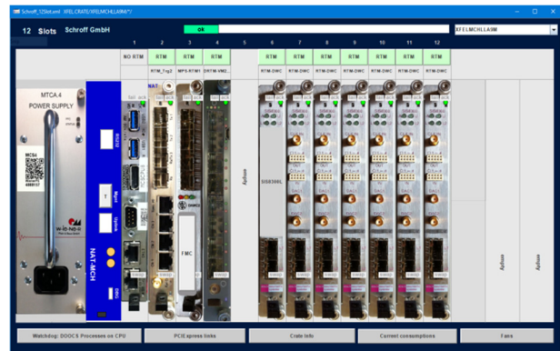
Figure 2: MicroTCA 12-slot crate view JDDD.
