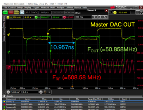
(b) F_{OUT} with phase offset +1,000 in the upper 11-bit of the phase-shift register.
