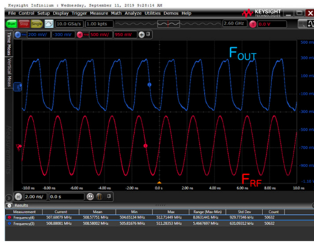
Figure 9: Observed 508.58 MHz F_{OUT} synchronized with F_{RF} ( =508.58 MHz).
