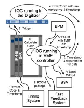
Figure 3: The original (before the upgrade) bunch length system process.
