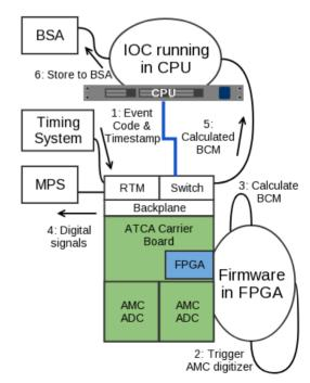
Figure 6: The upgraded bunch charge system process.
