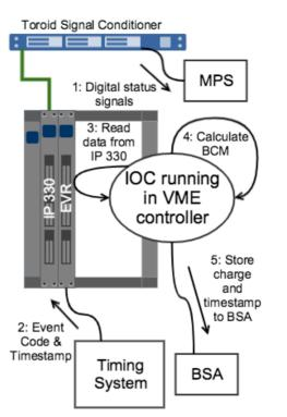
Figure 5: The original (before the upgrade) bunch charge system process.
