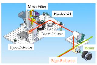
Figure 1: Optical structure of the bunch length system showing how the ER is reflected, split, and filtered before getting to the pyroelectric detectors. Reproduced from [1] with permission from the authors.
