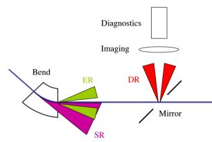
Figure 2: ER from bending magnet generating DR through a hole mirror. Reproduced from [1] with permission from the authors.
