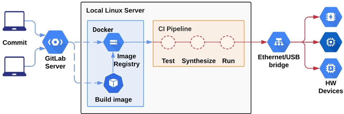
Figure 1: Hardware and software CI flow.
