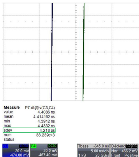
Figure 5: Jitter measured between 2 GFT1012: 4ps RMS.
