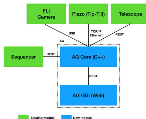
Figure 1: HARPS-N autoguider control architecture.
