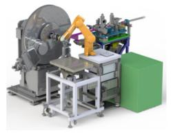
Figure 3: CAD representation of the robot to be integrated in the CRISTAL beamline.
