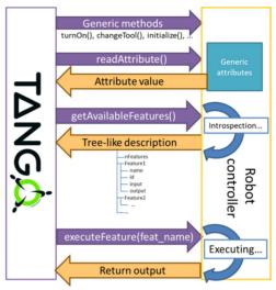
Figure 2: Software integration principle.
