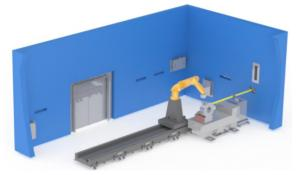
Figure 4: CAD representation of the robot to be integrated in the NANOSCOPIUM beamline, mounted on a translation axis.
