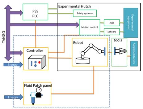
Figure 1: Architecture implementing an industrial robot at SOLEIL, and its interfaces.
