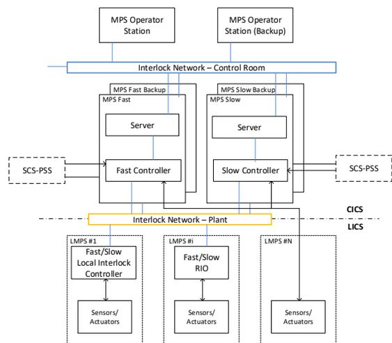
Figure 4: The MPS architecture.
