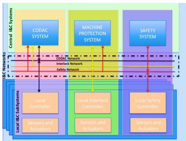
Figure 2: DONES I&C Systems: General First Level Architecture [10]
