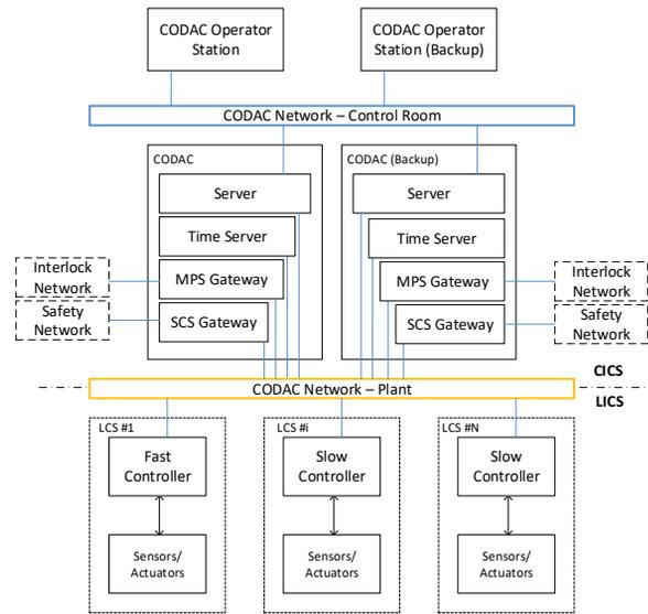
Figure 3: The CODAC architecture.
