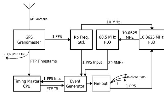
Figure 2: Synchronization and event generation machinery.
