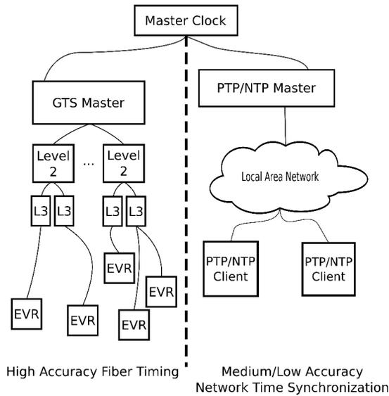
Figure 1: Simplified layout of FRIB's timing network.
