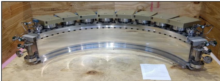
BNL 2D position-sensitive He-3 detector
