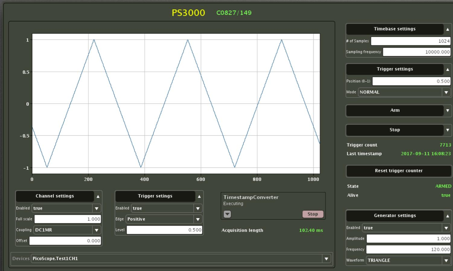
Universal oscilloscope panel implemented in Inspector using the FESA class as a data source.
