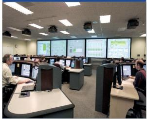
Automatic control of 192-beam shots is overseen by 14 operator stations
