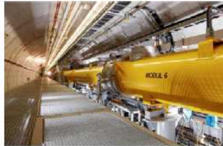
> TESLA type superconducting accelerating modules 1.3 GHz
