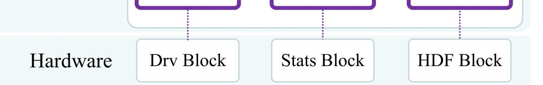
Each element in the areaDetector driver and plugin chain is defined by a Block in the Hardware Layer that defines the PVs it exports. The Device Block is then formed by composition from a single Controller and one Part for each child Block which contains the logic that shows how to use that Hardware Block within the current scan. This allows the external interface provided by PVs to be separated from small self-contained pieces of code that implement one particular type of logic.
