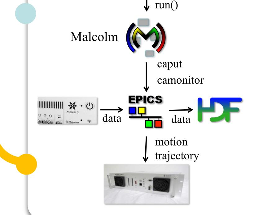
This means that it can take care of the variations in triggering schemes between different beamlines, and GDA only needs to pass high level scan parameters such as motion trajectory and exposure time down, rather than needing to know how all the underlying devices are wired up.
