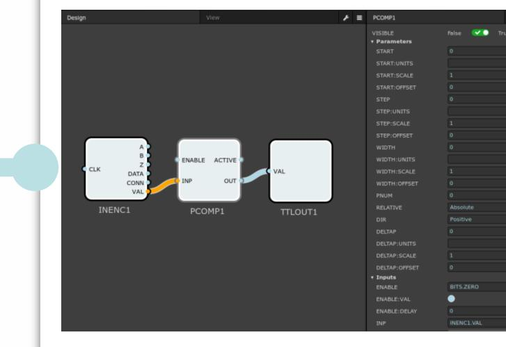
Websocket communications expose the structure of Malcolm Blocks via a JSON protocol over websockets. There is a client MalcolmJS library that is used to create a web GUI to allow configuration/load/save of Blocks from a web browser, like in a PandABox.
