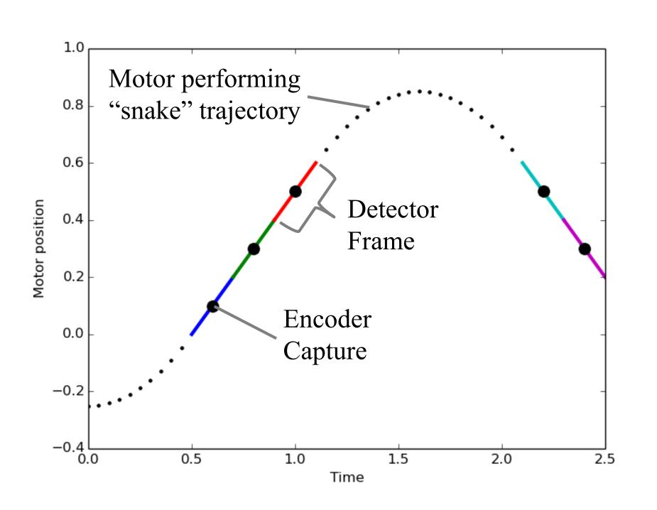
This technique increases the efficiency of an experiment by reducing the number of times a motor has to decelerate, settle and accelerate, effectively decreasing the scan dead-time
