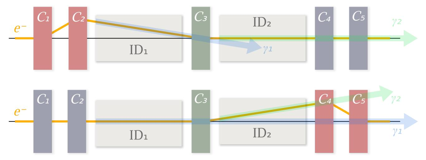
$C_1$  and  $C_2$  have zero field and pass the electron beam on axis generating a photon beam through  $ID_1$ , DC magnet  $C_3$  provides a kick that takes an off axis trajectory through  $ID_2$ ,  $C_4$  and  $C_5$  restore the nominal trajectory.
