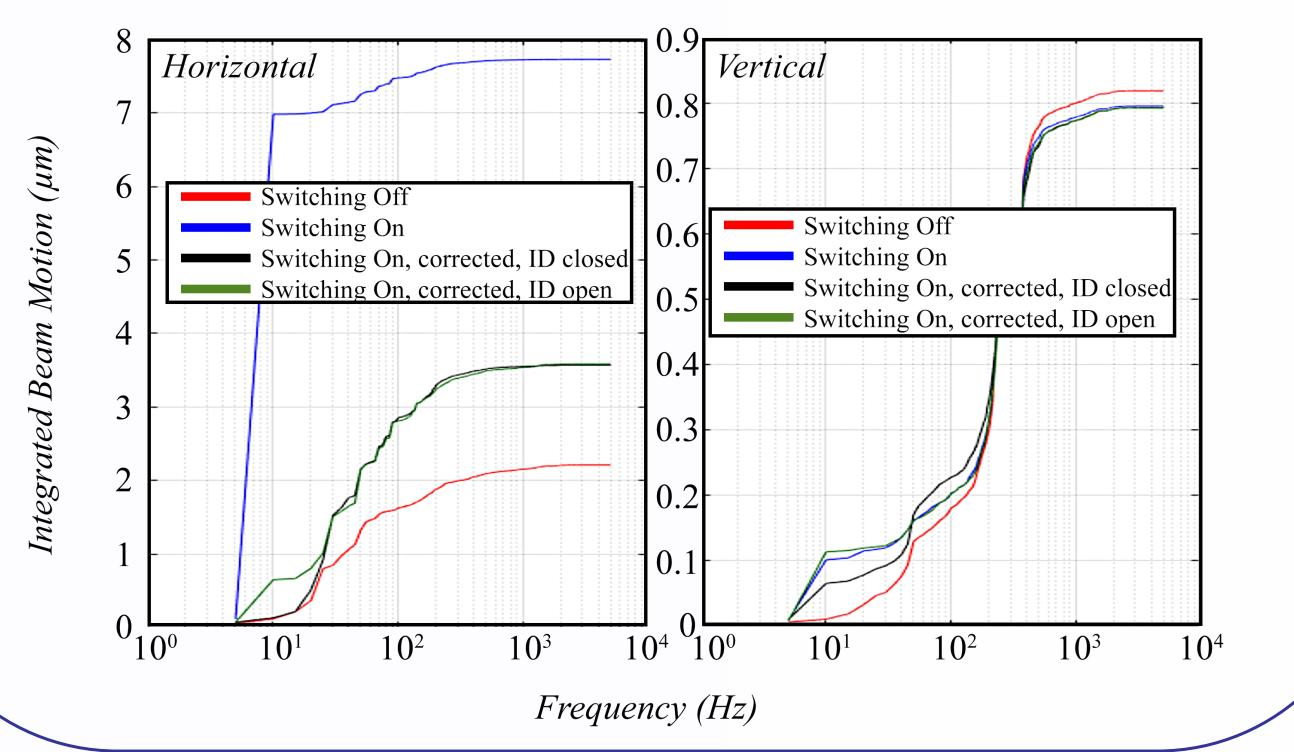
Result of the correction. Under ideal conditions the 10 Hz component is completely removed.
