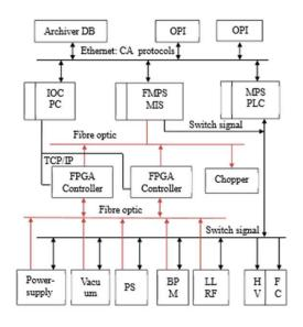
Fig. 2 Injector II MPS structure diagram
