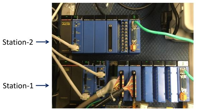
Interlock signal information transfer between two stations is performed through FL-net—an open network protocol used for interconnection between controllers.
