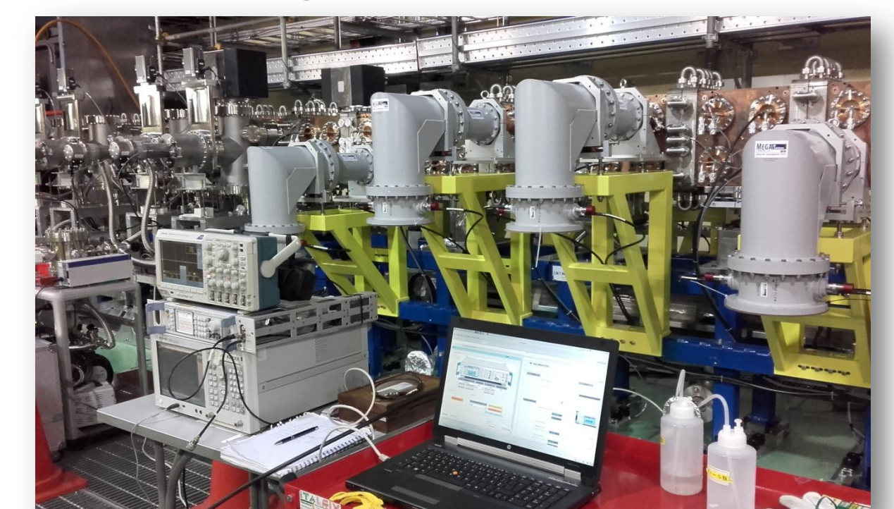
RFQ during RF cables calibration
