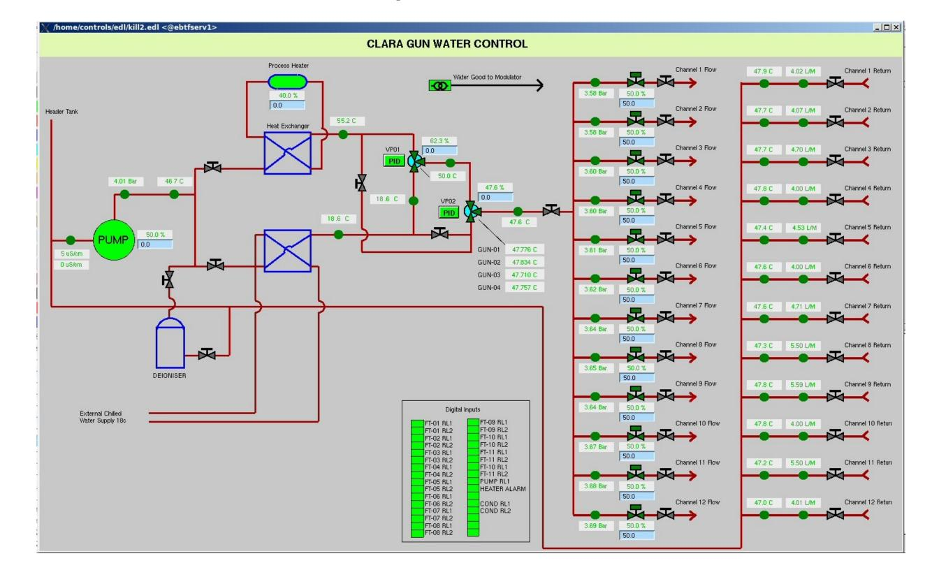
The gun temperature control operates by mixing two water temperatures close to the operating point. Two valves are PID controlled one produces a temperature just above the operating point which is then mixed with a manually set lower temperature to produce the fine temperature control.
