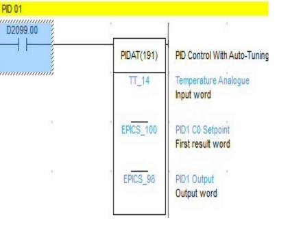
The function block appears to only have three parameters but memory space has to be reserved for setting all the other parameters and also for working memory internal to the routine.
