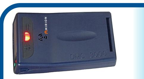
Operational dosimeters are Dosimetry provided by the Service at CERN. They are mandatory for everyone working in Limited Stay, High Radiation and Controlled Radiation areas [1]. The dosimeter displays the amount of dose and it has alarm functions when thresholds for dose or dose rates are exceeded. Before entering a hazardous area,
