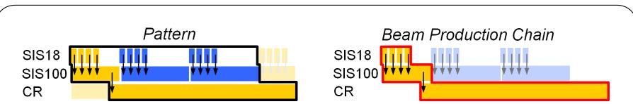
Patterns and Beam Production Chains as new concepts for scheduling beams, D.Ondreka, GSI.
