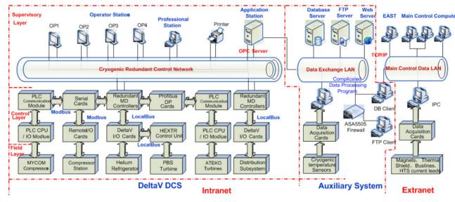
Figure 2: EAST cryogenic control system based on DelatV DCS.
