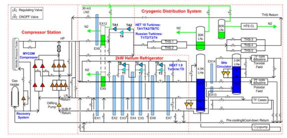
Figure 1: PFD of EAST cryogenic system.
