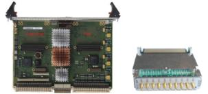
Figure 2: IOxOS cards (IFC1210 and ADC3111).
