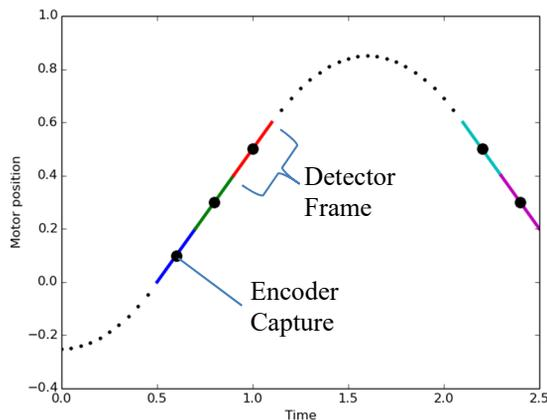
Figure 1: Detector frames synchronous with a motor undergoing a snake trajectory scan.
