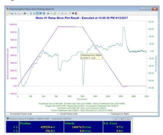
Figure 8: MFA-CC tuning ramp top, and executed motion at 140 cts/ms bottom, driven by GBLV 5A motor controller.
