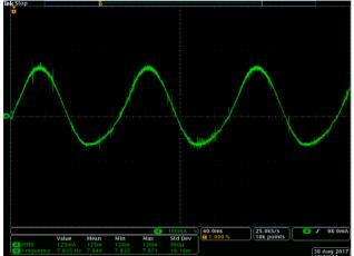
Figure 5: 125 mA stepper current trace, Ixx22=5, Ixx77=300, Ixx61=0.01.
