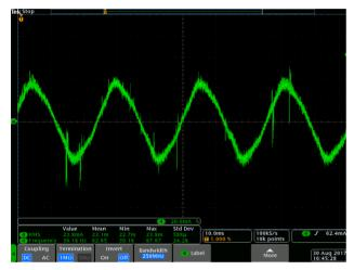
Figure 2: 45 mA stepper current trace. Ixx22=5, Ixx77=10, Ixx61=0.035.
