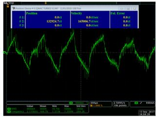
Figure 7: MFA-PP current trace, Ixx22=165 (rated speed), Ixx77=200, Ixx61=0.003; PeWin executed motion at 165 ct/ms.
