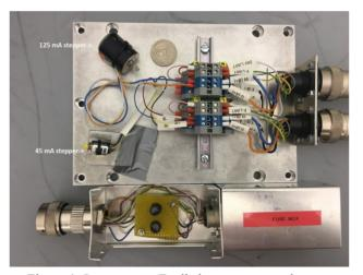
Figure 1: Low current Faulhaber steppers under test.
