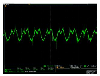
Figure 3: 125 mA stepper current trace, Ixx22=5, Ixx77=100, Ixx61=0.035.
