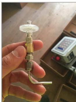
Figure 5: Detail of a filter for the micro-pipe input line.
