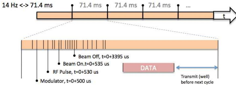
Figure 2: Machine timeline example.
