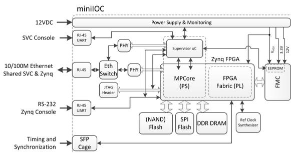
Figure 5: System architecture sketch of the miniIOC.
