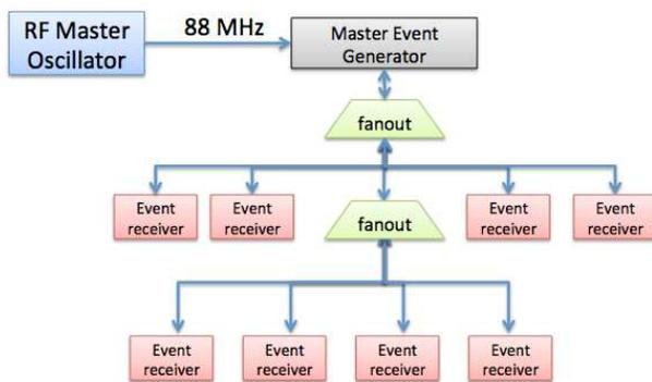
Figure 3: Timing distribution structure.
