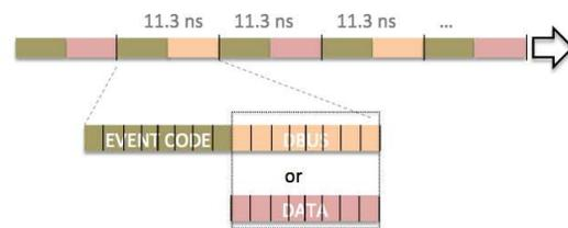
Figure 1: Frame structure of the timing system bit stream.
