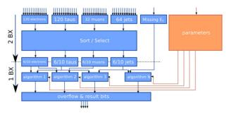
Figure 3: Block diagram of L1Topo execution. The input TOBs are sorted and truncated to reduce the combinatorial load put on the algorithms. Exactly 2 bunch group spacings (BX) of 25 ns are allocated to the sorting procedure.
