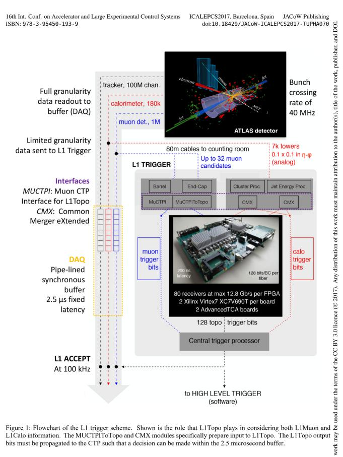
L1Calo information. The MUCTPIToTopo and CMX modules specifically prepare input to L1Topo. The L1Topo output bits must be propagated to the CTP such that a decision can be made within the 2.5 microsecond buffer.
