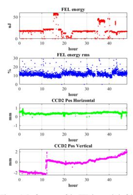
Figure 5: Performance of the FEL in a period of 48 hours with automatic optimization of the seed laser pointing. The third and fourth plots are the values of the sensors used for the optimization.
