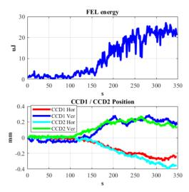
Figure 4: Automatic optimization based on four correlation minimizers working on the set points of the seed laser pointing feedback.
