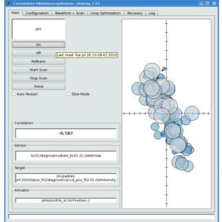
Figure 2: Graphical interface of the correlation minimizer. The spots on the right represent the relationship between the target (vertical axis) and the sensor (horizontal axis). The spots are big for the most recent samples and get smaller as the samples become older. In the example of the figure the correlation is almost linear and the correlation index is -0.587.
