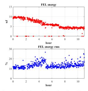
Figure 1: Typical decay of the FEL intensity and increase of the jitter in a time span of 11 hours. The jitter was reduced at the 5<sup>th</sup> hour by a manual re-optimization of the delay between the seed laser pulses and the electron bunches. The intensity could not be fully recovered because of an ongoing transverse misalignment of the two beams.
