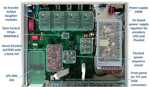
Figure 2: PandABox internal hardware top view.
