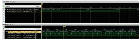
Figure 18: ILA captured detector data frames with PandABox.
