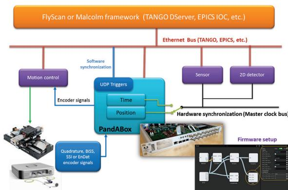
Figure 15: Continuous scanning synchronization with PandABox.
