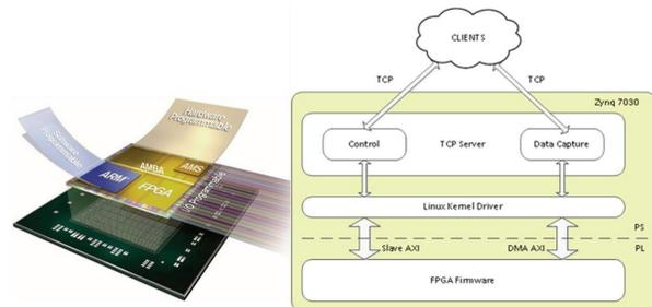
Figure 4: Zynq SoC firmware architecture.
