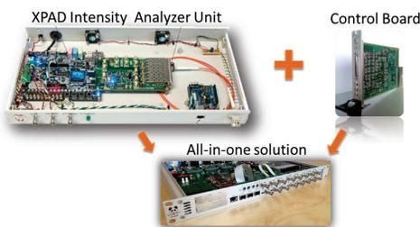
Figure 17: Fast beam-attenuation system upgrade with PandABox.
