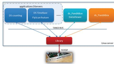
Figure 13: TANGO software architecture at SOLEIL.
