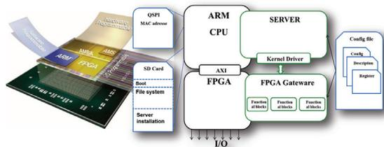
Figure 10: Flexible PandABox firmware architecture.
