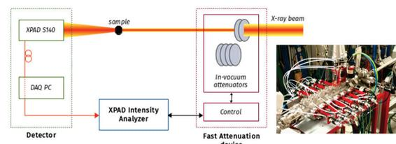
Figure 16: Fast Attenuation system on SixS beamline.
