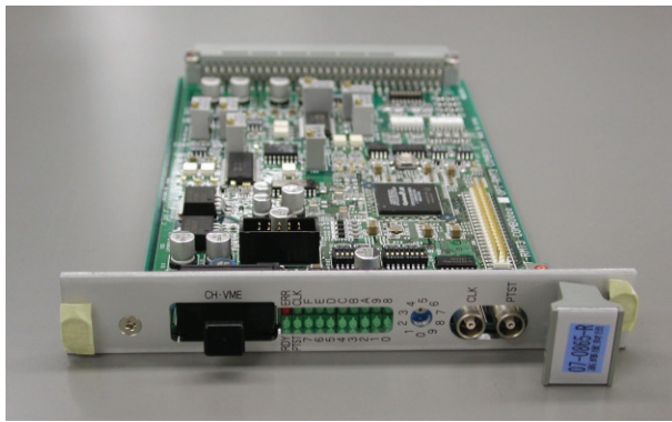
Figure 3: Photo of a kind of slave board called OPT-RMT COMBOdao used for controlling steering magnet power supplies at the booster ring.
