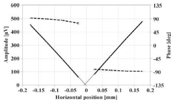
Figure 4: A typical graph of wire vibration amplitude and phase in quadrupole magnet. The amplitude is represented by solid lines. Thin lines show a linear function fit of the amplitude.
