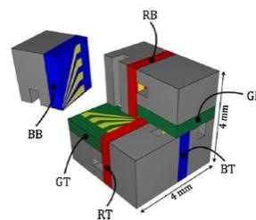
Figure 1: PSI 3D Hall probe structure. For clarity, pairs of 1D Hall probes sensitive to the same direction of the magnetic field are shown in the same color (blue: sensors BB and BT, green: sensors GB and GT, red: sensors RB and RT).
