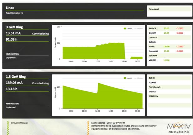
Figure 4: The main interface of the machine status application. Separated panels for both rings displaying the historic and instantaneous current, and status of the beamlines on each ring. The bottom part is devoted to status messages
