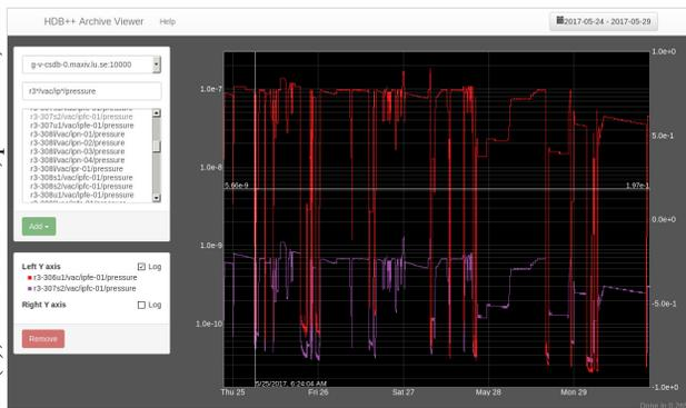
Figure 8: HDBPPViewer user interface. On the left, the user can filter within all the archived parameters and select the ones that will be plotted. The main view display the graphs, the user can zoom in and out and get basic information when hovering over the data.
