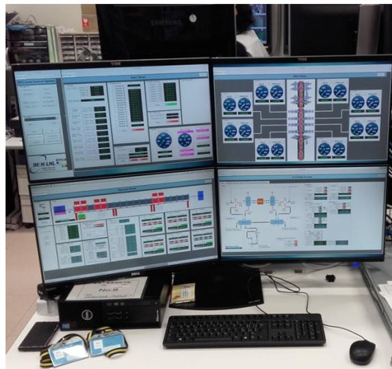
Figure 5: RFQ LCS Human Machine Interface installed in the control room.
