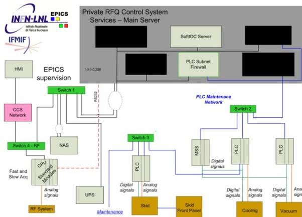
Figure 3: RFQ LCS Architecture for the final stage.
