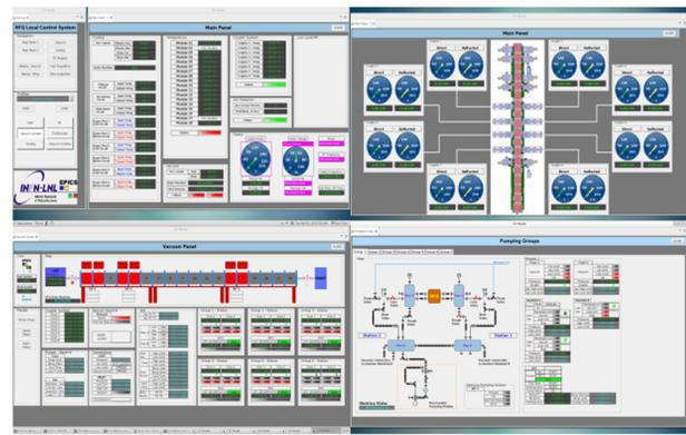
Figure 7: Control panels developed for the RFQ LCS.
