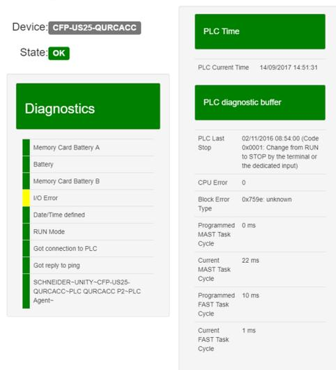
Figure 4: Fragment of the MARS UI showing the diagnostics information for a PLC.
