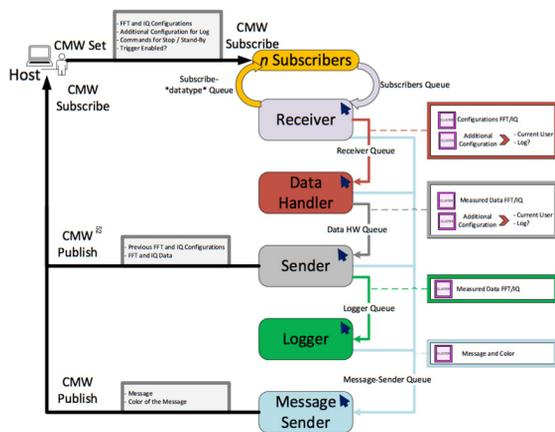
Figure 6: Target communication layers.
