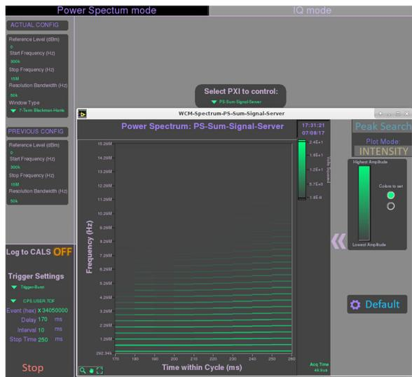
Figure 9: Example of a continuous power spectrum acquisition for an accelerating beam acquired by the WCM application.
