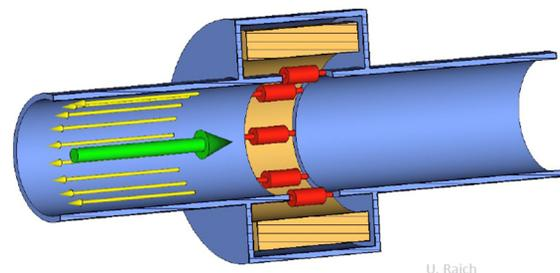
Figure 1: A schematic overview of a WCM. The green arrow represents the beam current, which is accompanied by its own image current (yellow arrows). A set of resistors (the red cylinders) generates a measured voltage. Ferrites, which are electrically insulators, (light brown section) forces the image current to flow through the resistors.
