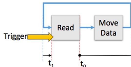
Figure 8: Illustration that indicates the dead time from  $t_0$  to  $t_1$  by iterating for the next power spectrum read.
