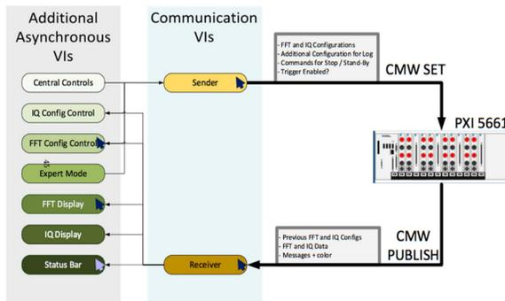
Figure 5: Host communication layers.
