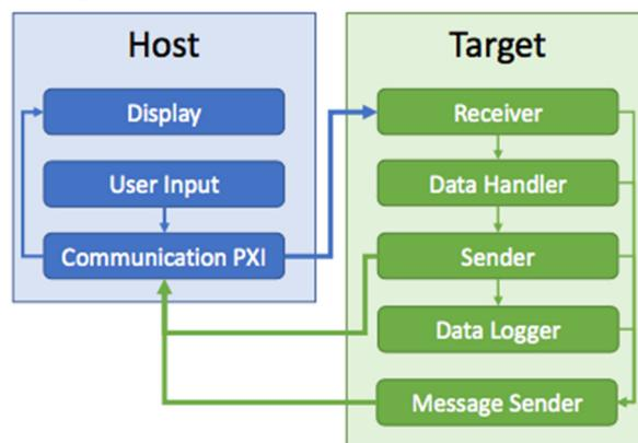
Figure 4: Simplified WCM application layers.
