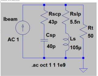
Figure 1: Simplified Passive Current Transformer
